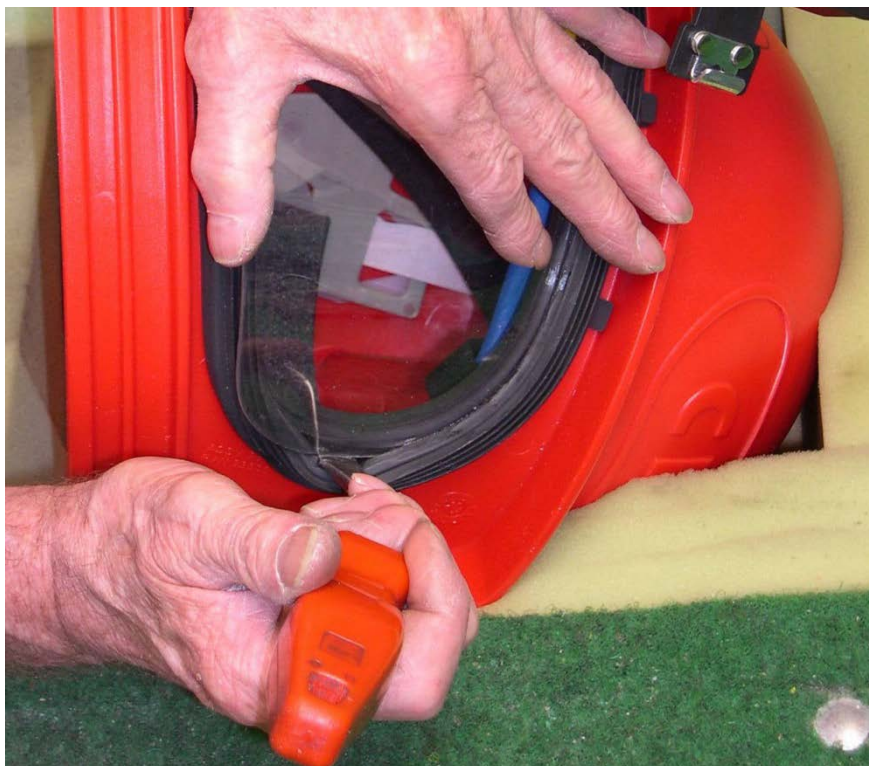
Figure 3: Replacing the inner lens using the installation tool
