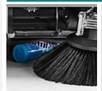
The flap fitted to the front of the machine is activated from the driver's position and allows the main brush to pick up bulkier debris
