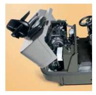
Just the checking of the oil or changing the filters for instance, in the motorised version, is now very easy. In the B version the box that houses the electrical devices is positioned centrally so it is quick and easy to check the devices and the level of the fluid in the battery elements. A battery box can be installed with a capacity of up to 480 Ah C5 (CS90B-CS110B version)
