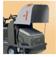
A fabric bag filter, with a large filtering surface -7 sq.m (CS80) - 8 sq.m (CS90-CS110) - lasts a very long time and ensures excellent results even in environments where there is a lot of fine dust thanks to the powerful filter shaker. The filter is easy to remove without the use of tools, to check or replace it. No maintenance is required thanks to the periodical use of the electric filter shaker. Filters in fabrics for specific applications are available upon request
