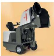
**Discharge height: 1.4 m** The front box for collecting dirt has a capacity\* of: 190 l. (CS80) - 220 l. (CS90) - 270 l. (CS110) and is lifted by a 2-piston hydraulic system operated by the handy control where the driver sits. Vacuuming is operated by a hydraulic motor
