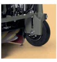
Besides reducing mechanical stress the large diameter wheels also make working more comfortable. Their sturdy support helps keep operating characteristics always the same.
