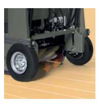
The central brush is the floating type and self-adjusts to keep in contact with the ground all the time
